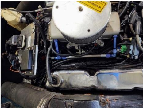
Your Optimum Marine AFI system may have been ordered with a 4 bbl. throttle body. The 4 bbl. installation is slightly different than the 2 bbl. units. A 4 bbl. TBI unit will look much like a 4 bbl. carburetor you may have seen with the injectors underneath what would normally be a fuel bowl. These units are true 4 bbl. as they work off the front two barrel's/injectors and bring the rear two injectors in as the secondary throttle plates open.
