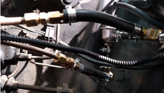
and plugged allowing the fuel to be pressurized through the throttle body to the regulator. On the end of the regulator is the return and opposite that end a vacuum line is attached which varies the fuel pressure, the same as the 2 bbl. application.
