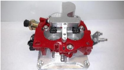
Connect the fuel line to the backside of the throttle body. This is an AN type or barbed pipe thread fitting and is sufficient for the pressures encountered with the fuel injection system.
