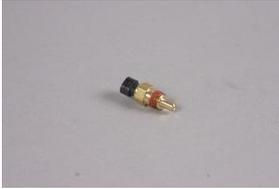
sensor or anywhere on the engine side of the thermostat. Connect the two-wire connector when installed. Ensure that there are no coolant leaks from the threads of the sensor. It is also important that a continuous flow of coolant is present at the tip of the sensor or a false reading and engine damage can occur.
