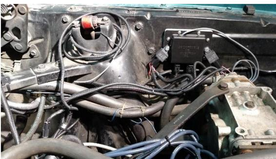
This Optimum EFI fuel injection system can be configured for full ECM control of the spark advance. A distributor module is mounted inside of a high temperature plastic box and mounted to an aluminum base plate for Ford applications.
