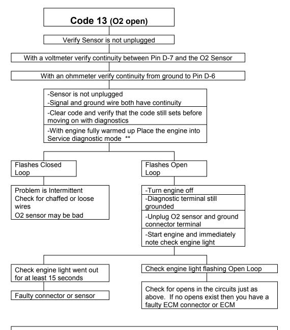
\*\* Service diagnostic mode is entered the same as Engine Off Self Test. Ground out Pin A and B on the ALDL connector with the engine running. Rapid flashing (approx 1/2 - 1 sec interval) is open loop. Flashing at a slower rate indicates closed loop.
