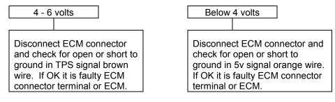
33. High voltage (low vacuum) at MAP sensor, sensor could be unplugged.
