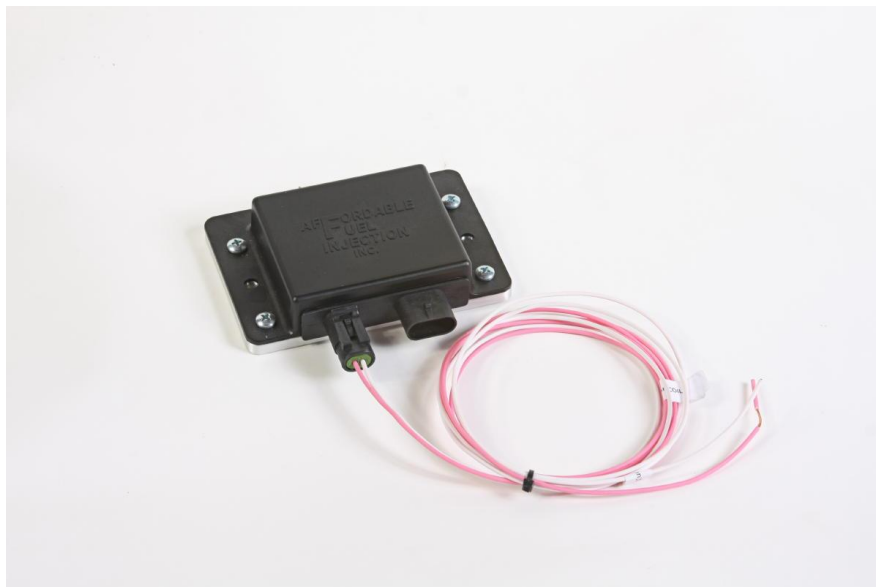
Distributor module connections. Pink - 12v white to coil neg.
