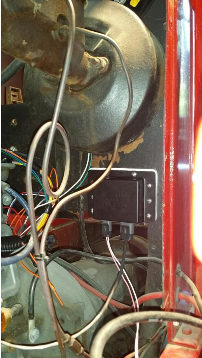
Distributor module connections. Pink - 12v white to coil neg.
