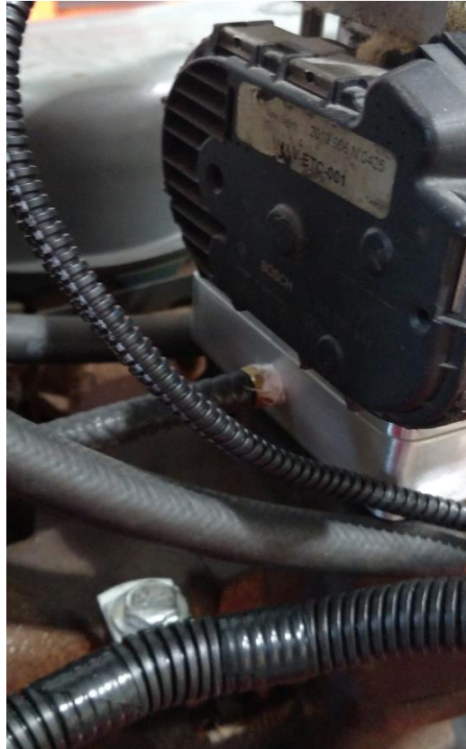
MAP sensor vacuum line attachment
