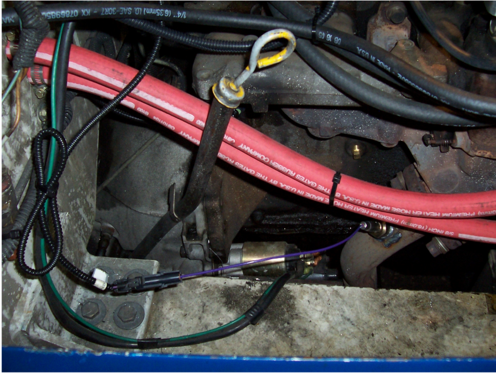
Typical O2 installation when tapped hole is not available in the exhaust manifold. An 18mm hole can be drilled and tapped into the standard O2 location in the exhaust manifold.
