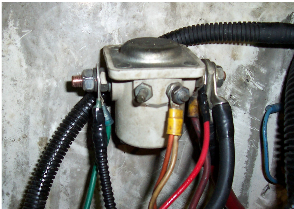
Solenoid connection, crank wire on crank side of starter solenoid and Battery power to the other side.
